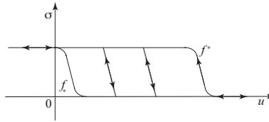
**Figure 2.** Generalized stop operator
